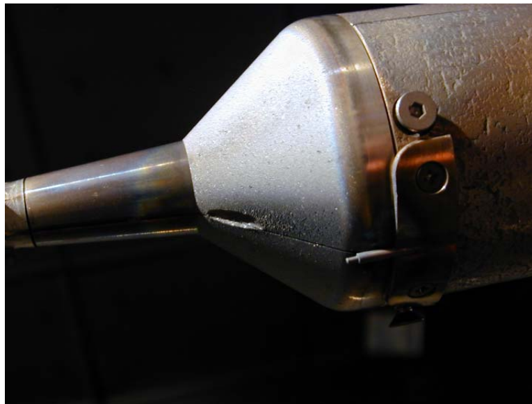
Figure 22: The extremely high heat load in the boundary layer separation zone resulted in local melting of the SICTO surface.
